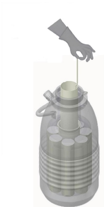
Figure 1: Inserting or removing canisters
