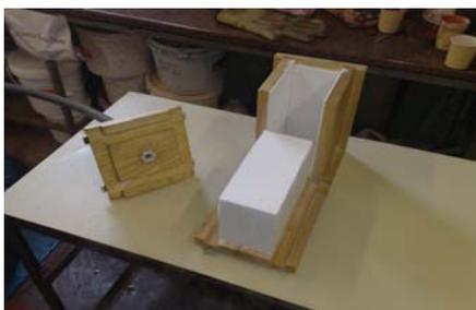
5. Open dry ice block machine by loosening latches and folding down sides. Remove block for use or storage. **Caution: always wear protective gloves** when handling dry ice; **can cause burns and frostbite.** Blocks can be stored in Dilvac Dewar Flasks.
