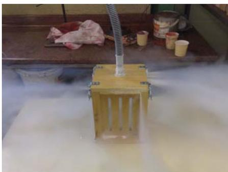
4. **Vapour will discharge through vertical filter slots as dry ice block is forming.** When vapour discharges from space between lid and body of machine (and sound changes), the dry ice block is formed. Immediately close cylinder valve.
