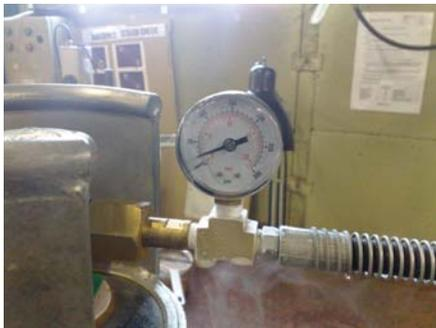
3. Open CO<sub>2</sub> cylinder valve **no more than 1-2 small divisions** on inner scale (0-20) of gauge. This gives maximum number of ice blocks and does not waste CO<sub>2</sub>. Be sure vapour escaping from vents of machine does not carry snow solids. If there are, close down valve slightly. After ice builds up in machine, speed up process by opening the valve another degree or two. If needle reaches 10 on inner scale turn valve off.
