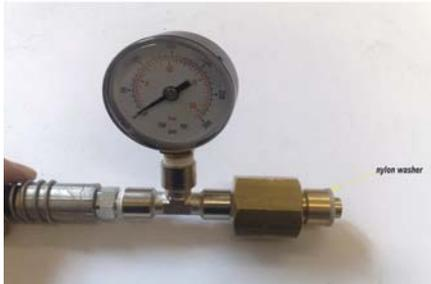
1. Firmly connect machine hose to CO<sub>2</sub> cylinder. Use plastic washer supplied for inside of hexagonal nut that attaches to cylinder.
