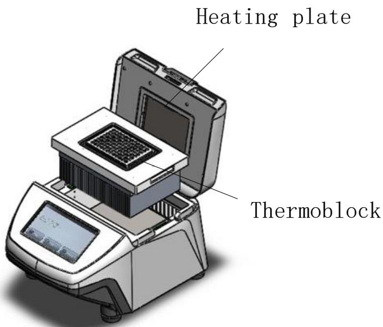
**Heating plate:** Heat for the heated lid
