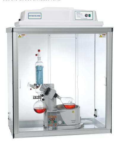
The clear polycarbonate shell and horizontal sliding doors offer excellent visibility and ease of access for monitoring the enclosed equipment. The LabPartner rotavap enclosure is only 24 inches deep and 38 inches wide, taking up minimal space within the laboratory.
